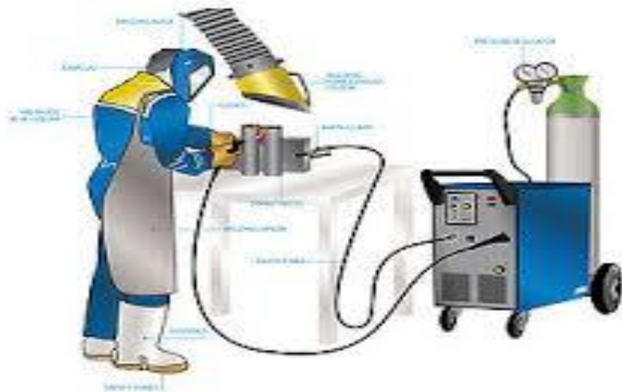
Correct and safe electric welding station
